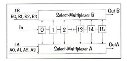
Internally, it is equivalent to a 16-tap delay line with two multiplexers for selecting which taps are routed to the outputs. Each multiplexer has a 4-bit parallel input to select the required tap, so one byte of data could fully program the device.
